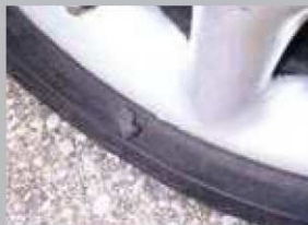
Tyres with impact damage e.g. 'kerbing', bald tyres and those below 2mm tread depth are unacceptable.
